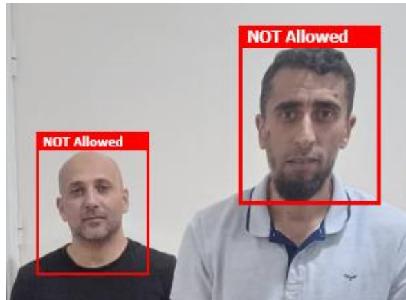
Figure 10: The system displays a "Not Allowed" message when more than one student is in front camera
